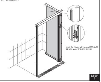
Install the moving door leaf, align the upper and lower rail grooves of the open door leaf, Then install the moving door leaf into the open door leaf.
