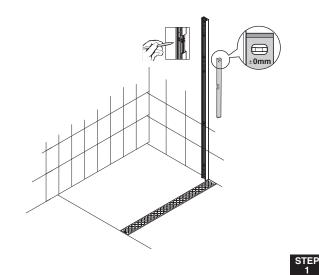
Assemble the door frame, note that the second rail needs to be connected by magnetic (door-closing) hinge slot. 组装门框框架,注意第二导轨段需靠磁吸 (关门) 立柱侧锁接。
