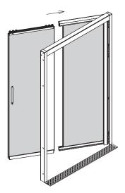
Adjust the adjusting screw in the wall material to make it level. Pay special attention to the level of the butt end of the upper rail. Then lock the end of the first rail. 调节墙材内的调节螺丝使之水平,特别注意上轨对接端头要水平。然后再锁好第一导轨端
