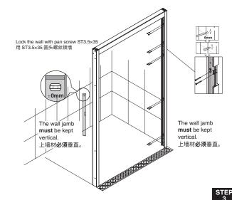
Install the side-hung door leaf, lock the hinge on the side-hung door leaf with screws in the hinge column slot. Install the waterproof tape (water retaining edge facing outward) and adjust the level.
